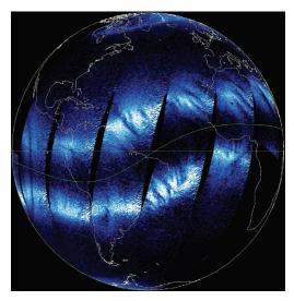
forecasting using solar measurements and models. High-resolution modeling capabilities, with horizontal resolution of ~10km, are also necessary to capture small-scale and impactful space weather events, such as the onset and development of ionospheric equatorial plasma bubbles, as shown in the ultraviolet image taken by the GUVI instrument on board the NASA TIMED satellite (as the dark streaks across the bright ionospheric background).
